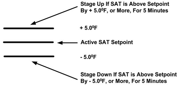
**Figure 7: SAT Control Band**
