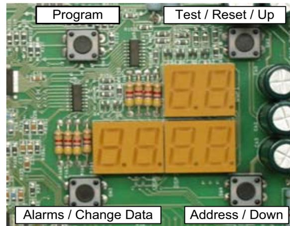
**Figure 2: Simplicity<sup>®</sup> Controls Push Buttons**
