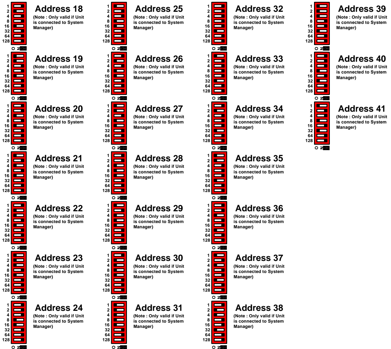
Figure 2: Address Switch Settings for YK-PEC1001-0 Units Connected to System Manager
